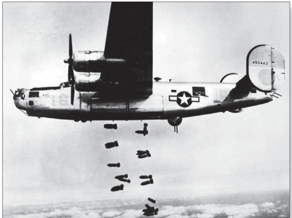
Brought into war service in 1943, the B-24 was a rugged heavy bomber, but the placement of its fuel tanks throughout the upper fuselage and its lightweight construction made it vulnerable to battle damage and a tendency to catch fire.
